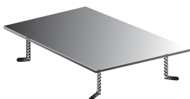
Foundation plate on which the Drive Unit is placed.
